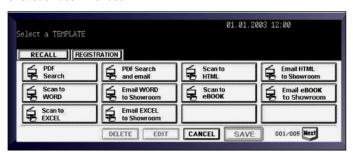
e-BRIDGE Re-Rite allows for automatic document scanning, optical character recognition, format conversion and document routing with a touch of a single button from the e-studio MFP control panel.
