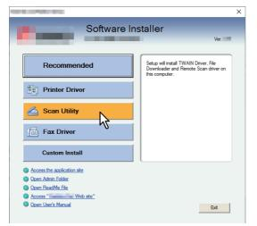
4 Confirm the list of the software to install, select the port to connect to this equipment and click [Install].
