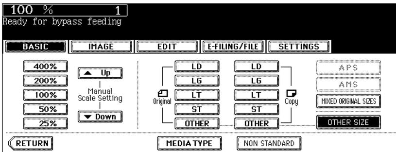
**6** Press the envelope size button corresponding to the envelope placed on the bypass tray.
