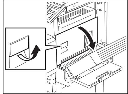
**4** Rotate the green knob as indicated by the arrow toward the inside and remove any misfed paper.
