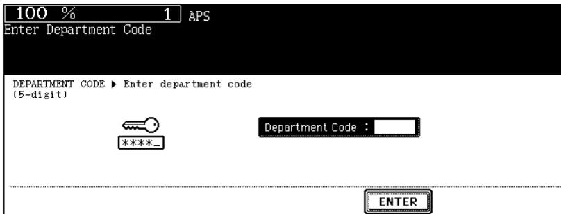
Key in a department code (5 digits) previously registered and press the [ENTER] button. The menu will switch and the equipment will be ready to be used.
