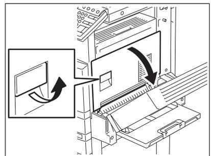
**9** Open the transfer cover to take out the transfer charger cleaner from the front pocket.
