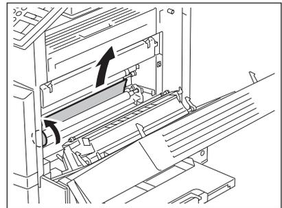
**5** Return the jam releasing cover, the automatic duplexer and the bypass tray to the original positions.
