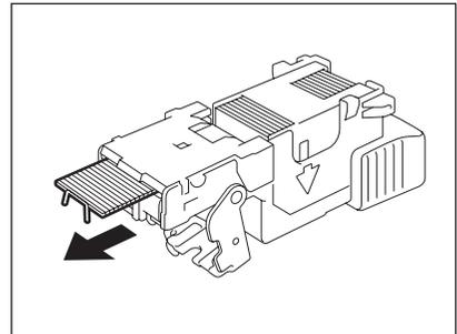
**5** Hold the knob and raise the guide, and then return the guide to its original position.
