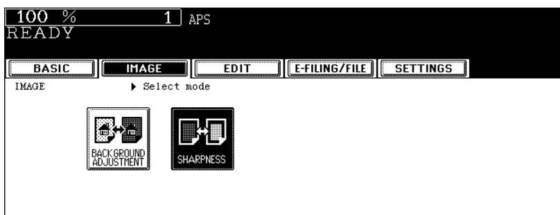
**4** Press the [SOFT] (or [SHARP]) button to adjust the sharpness, and then press the [ENTER] button.
