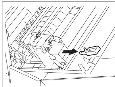
**10** Wipe the transfer charger wire properly with the transfer charger cleaner.
