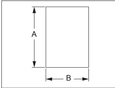
When “B” is longer than “A”, it is called “placing the original in a landscape direction.”
