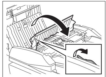
**5** Raise the guide plate under the transport guide, and then remove the original under the guide plate.
