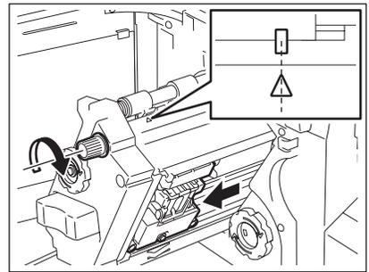
**3** Holding the both sides of the green area of the staple cartridge, take out the cartridge.
