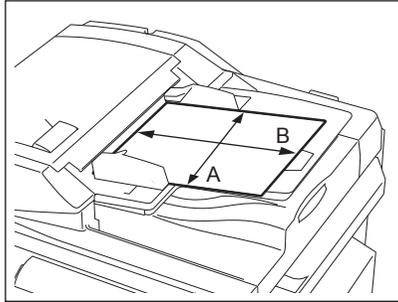
When “B” is shorter than “A”, it is called “placing the original in a portrait direction.”
