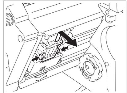
**4** Holding the knob on which the blue seal attaches, raise the staple cover.
