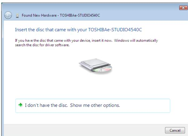
When you insert the Install Disc into the disc drive, Software Installer may launch automatically. In this case, click [Exit] to close it and continue the operation.
