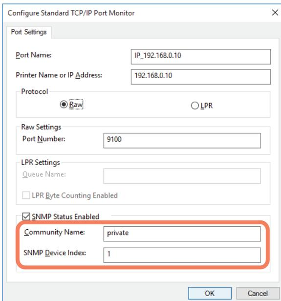
The Read Community Names must be the same in your TOSHIBA MFP and the [Ports] tab. Make sure that the value of [SNMP Device Index] in the [Port Settings] tab is set to "1".
