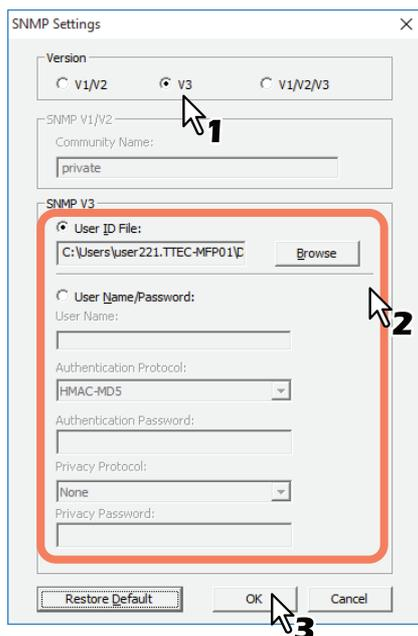
\* When SNMP V1, V2, and V3 are configured for your TOSHIBA MFP, perform both of the above settings.
