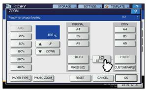
3 Press the button of the same size as the paper you placed on the bypass tray.
