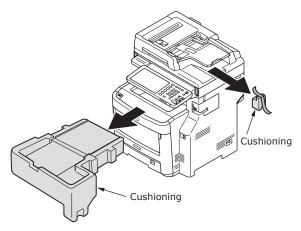
(2) Remove the protective tape from the back and sides of the machine.
