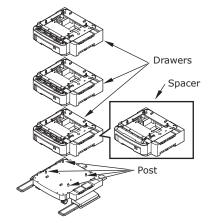
(2) Fix the drawer with the jointoption and tighten the screws with the screw-knob.
