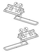
(2) Put the bottoms of the anti-tip feet (both sides) on the floor, align the sides to the cabinet and tighten them with the two screws each.
