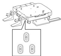
Attach the screw in the middle of the oval cutout and tighten the screw.
