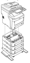
(2) Fix the additional drawer unit with the joint-option, and tighten the screw with the screw-knob.
