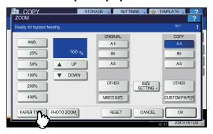
12 Press the button of the same paper type as the paper you placed on the bypass tray. Then press [OK].
