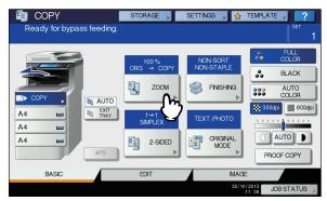
10 Select the same size button under "COPY" as that of the paper you placed on the bypass tray.
