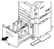
3 Adjust the paper guide and paper stop to fit the paper size, and make sure they are secure.
