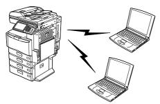
In the Ad Hoc Mode, client computers can access to the equipment directory through a wireless network without an Access Point. The Ad Hoc Mode is not suitable for the wireless network that many computers are connected, however, it is easy to establish the wireless network because the Access Point is not required.
