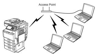
In the Infrastructure Mode, client computers can access to the equipment through a wireless network via an Access Point. The Infrastructure Mode is suitable for the wireless network that many client computers are connected at the same time. The Access Point will be required to establish the wireless network in the Infrastructure Mode.
