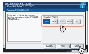
Select the low transmit power if you want to limit the area that the wireless communication is enabled. If you do not have to limit the area, select [100%].
